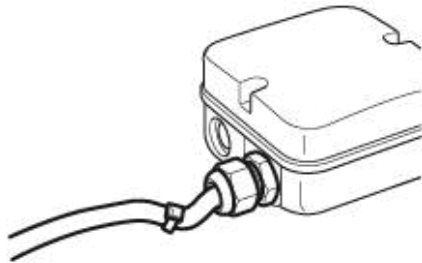
Fig. 1: Fan installed horizontally, routing of the cable as a U-shaped loop (illustration as example).
